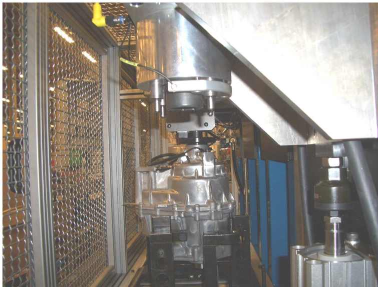
Vehicle gearboxes being automatically assembled leak tested and filled with oil ready for fitting to the vehicle
